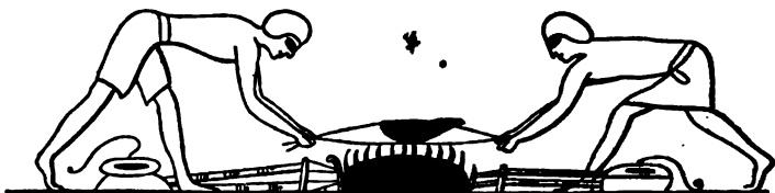
No. 104. Egyptian Bellows in use before the Exodus.
